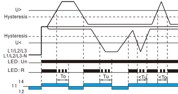
To: Overvoltage threshold tripping delay.
